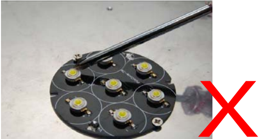
Figure 7. The screw driver strikes the LED
